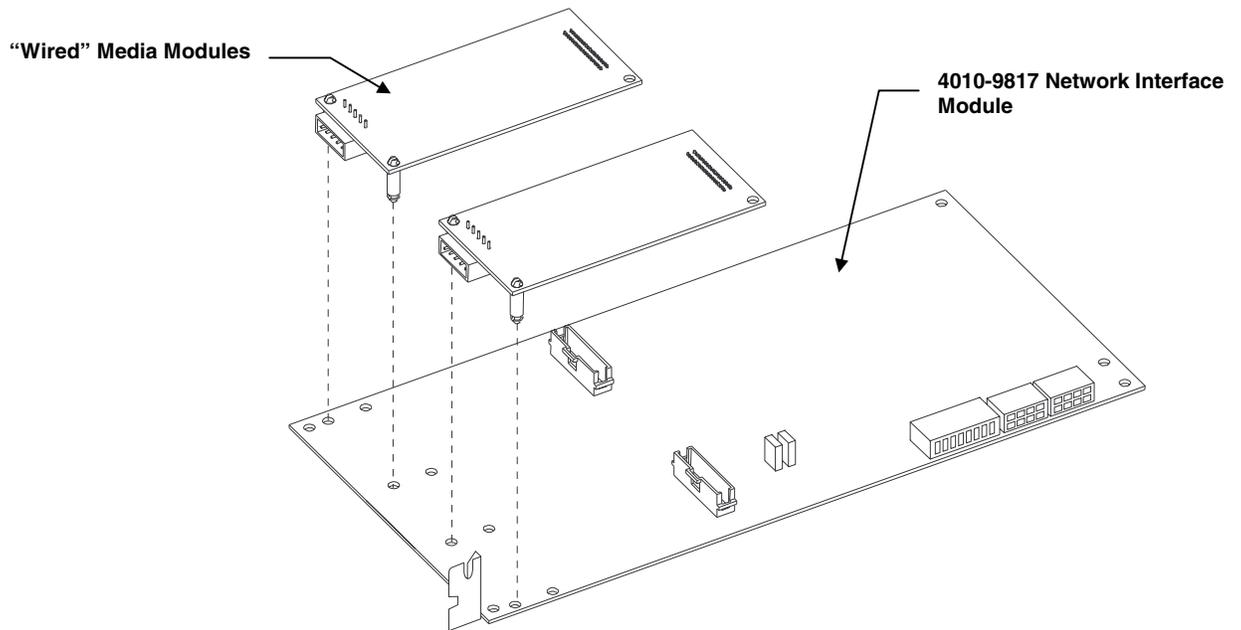
**Figure 1. Modular Network Module**
