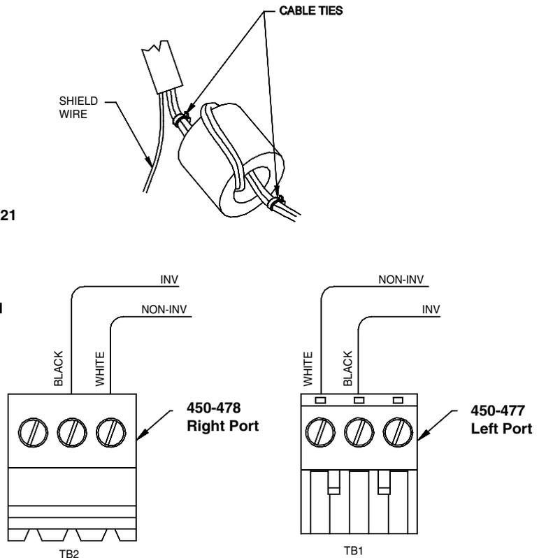
Figure 8. 4010-9821 “Wired” Media Network Wiring
