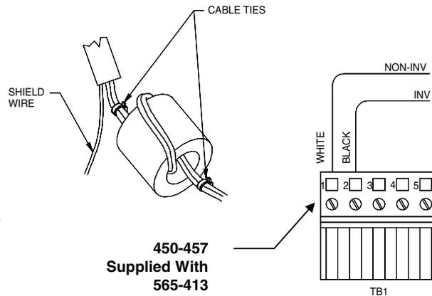
Figure 6. Network Wiring and Ferrite Bead Installation
