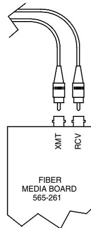
Figure 7. Installing Fiber Optic Cables
