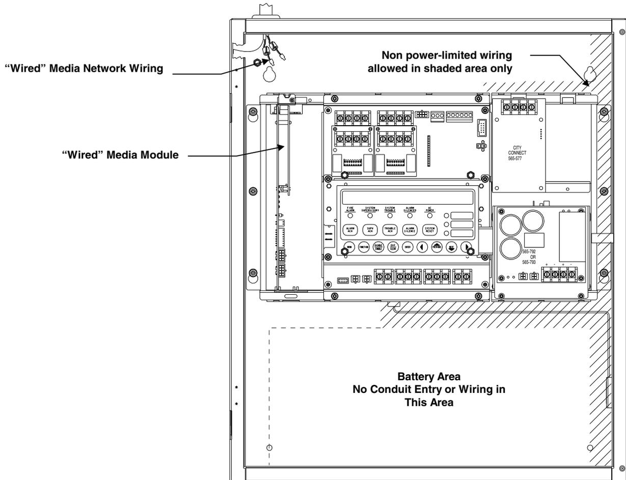
Figure 5. "Wired" Media Network Wiring
